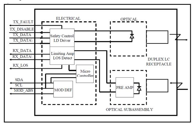
**Transmitter Section-** The Laser driver accept differential input data and provide bias and modulation currents for driving a laser. An automatic power-control (APC) feedback loop is incorporated to maintain a constant average optical power.1310 DFB in an eye safe optical subassembly (OSA) mates to the fiber cable.
